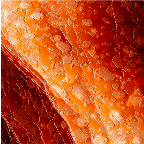
Figure 4. 750 nm \times 750 nm STM image of graphene islands on Ru(0001) stepped surface. The image was taken with a sample bias voltage of V_s = -0.9 V and a tunnel current of I_t = 0.1 nA. The topographic image is numerically differentiated along the X direction.
